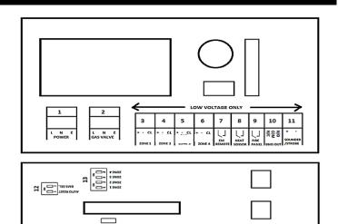
Note: Terminal blocks are plug/socket type and may be removed to ease wiring.
