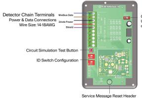
Chain Termination Resistor Used to select the first and last device in the chain
