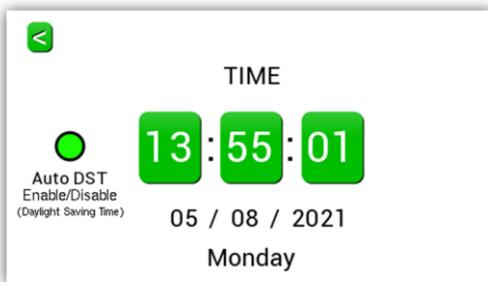
Press the time, date, or Auto DST section to adjust. To return to menu, press the back arrow.
